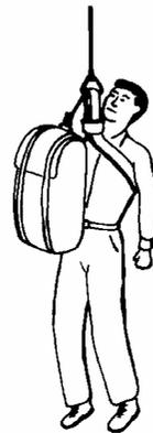
**Fig. 6.3 Winching with a chest sling**
